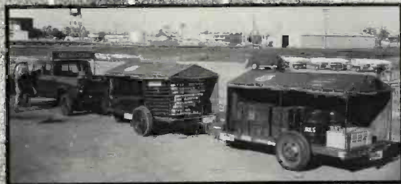
Trailer with side curtains rolled up ready for use. Side curtains should also be left up in hot weather to keep contents from being damaged by excess heat. Note neat arrangement in second trailer for carrying ammo and containers for loose links and rounds.
